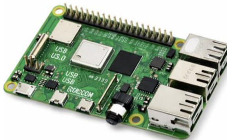
Fig.2. Raspberry Pi 4 Model B
